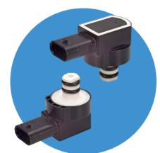
A combination of robustness and precise measurement means that these pressure sensors are increasingly used in low pressure applications. An integrated temperature sensor provides a temperature signal for the system.
