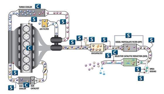
Exhaust after-treatment in particular requires sensors for a wide field of applications.
